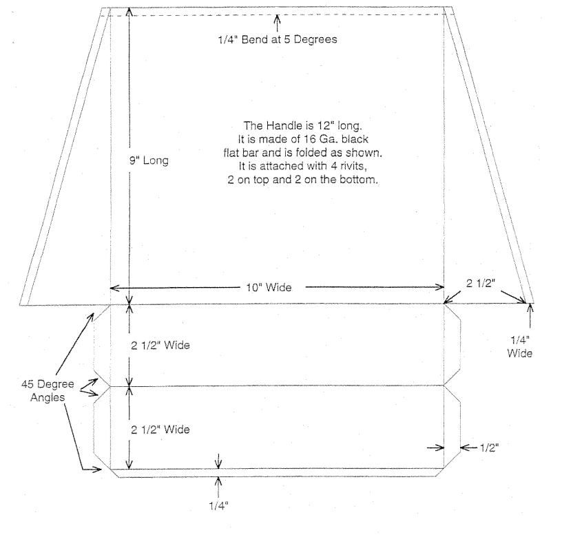
Use a piece of 26 Ga. Galvanized sheet metal 16" by 16" for this project
