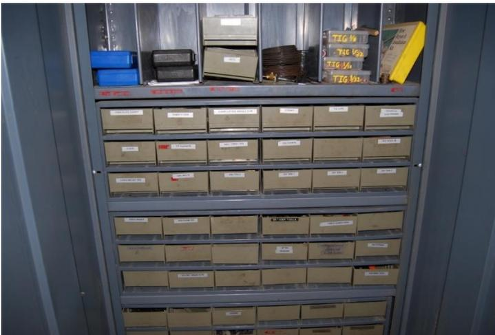
Many types of commerical bins are availabe for storing fasteners and small parts. They should be clearly labled. Fasteners (nuts, bolts, and screws) organized by size and type. Note:
