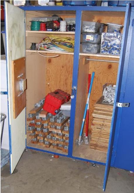
An example of materials for a specific project (electrical) being stored together. The cabinet is only opened when the materials for the project are needed.
