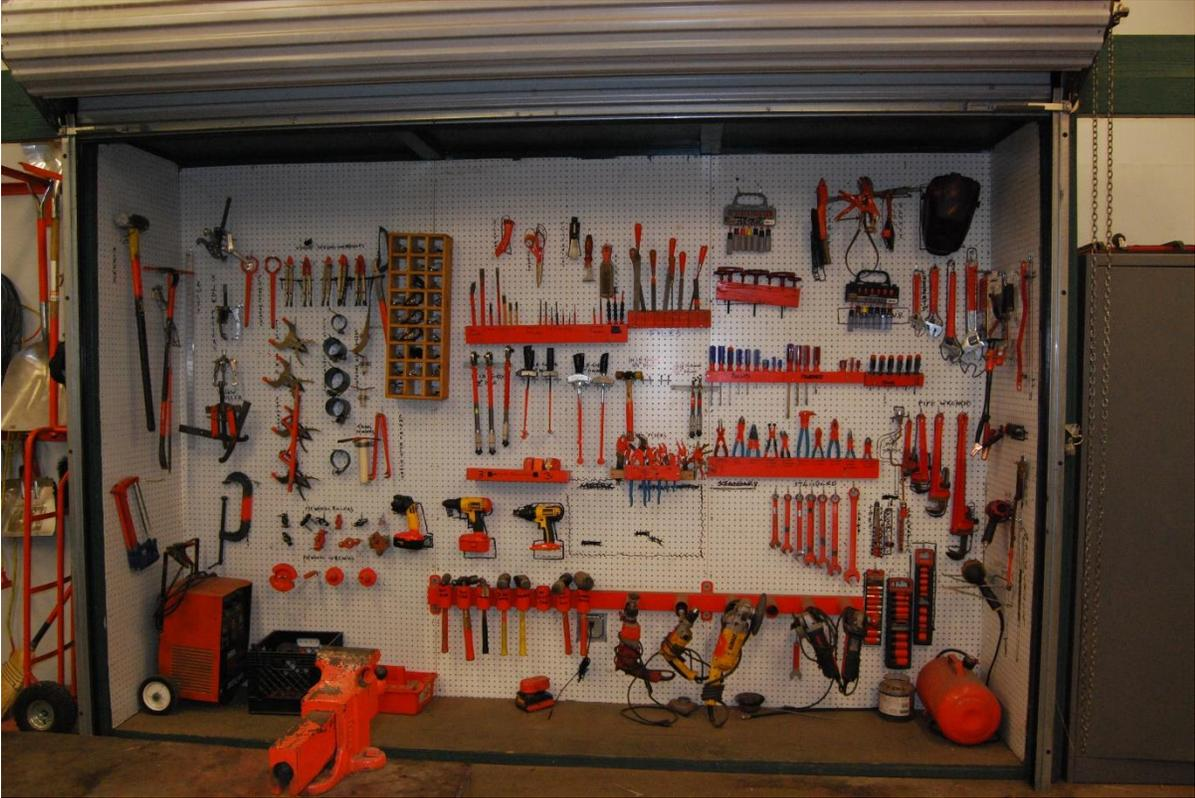
Use of pegboard for storage. The advantage is that you can use purchase brackets and easily move items around. Note the use of a roll up door for security and some custom brackets.
