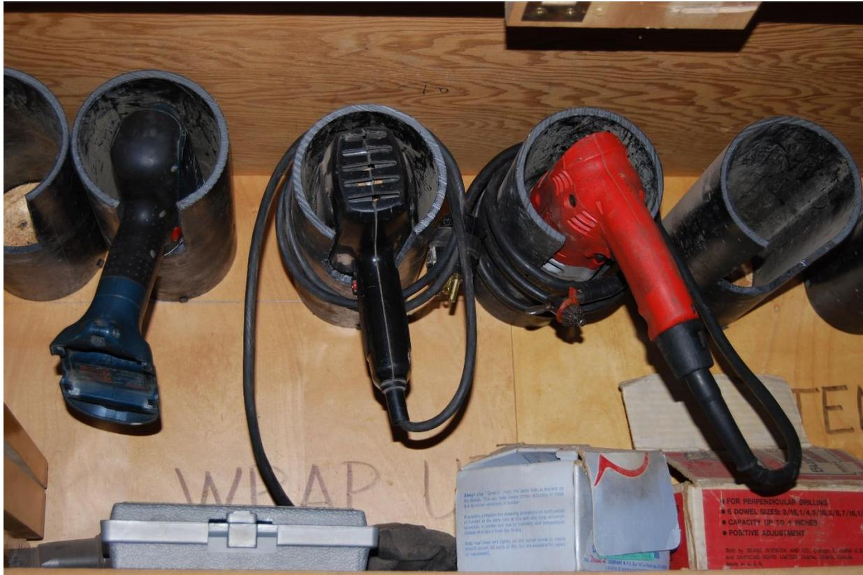
Portable drill holders made from ABS pipe. Note the storage of the cords.
