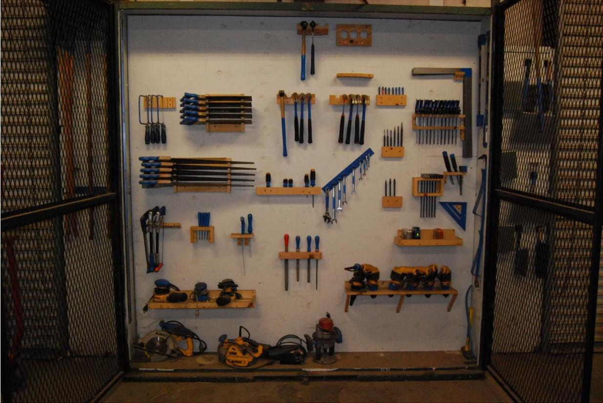
Cabinet with wood brackets and expanded steel doors.
