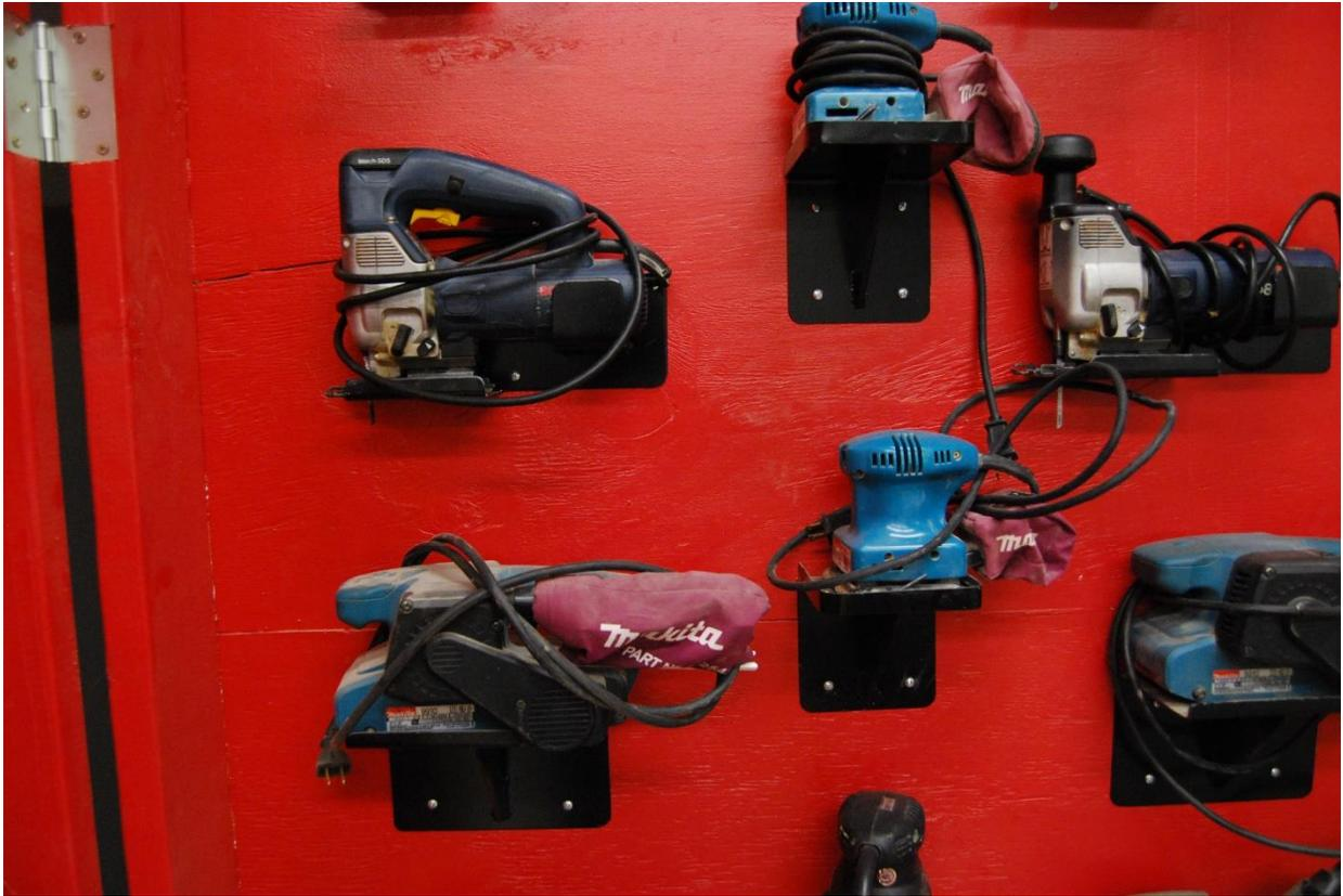
A good example of custom tool holders. These were plasma cut then bent in a brake.
