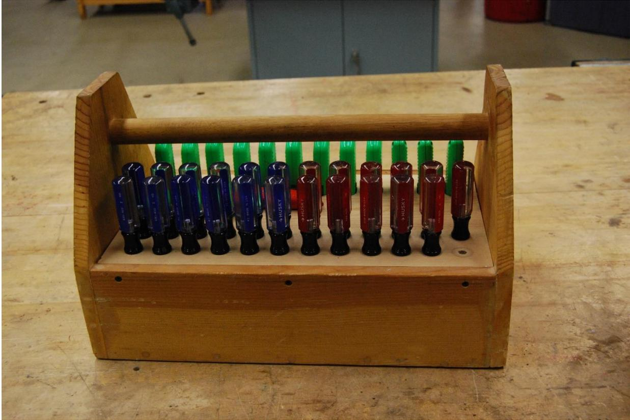
An example of “caddy” storage. Very useful for specific projects. In this case electrical. Caddy is stored away when not needed. Easy to inventory as every slot should be filled. Hint: If you are using this type of storage and have a missing tool place tape over the slot until it is replaced.
