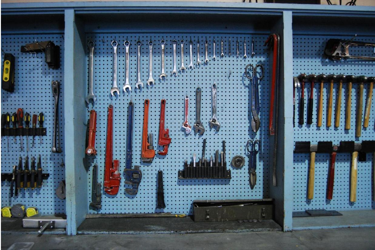
Pegboard can be used to hang tools. It is flexible. Hooks can be glued with a hot glue to prevent falling out and tool outlines can be drawn around tools.
