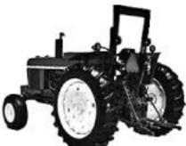
Tractors will start in gear if normal starting circuitry is bypassed. Start the engine from the operator's seat with the transmission in park. Do not start the engine by shorting across starter terminals. **Never** start the engine while standing on the ground.
