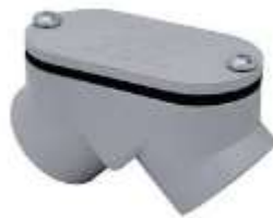
PVC Pull Elbow Used to make 90 degree bends and has removable cap for splicing or pulling wire. Glues to PVC conduit. Types denote the location of the cover (e.g. LB, LR)
