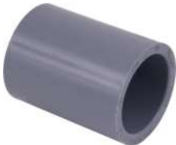
PVC Conduit Coupling Used to connect PVC conduit, must be glued and once connected cannot be removed.
