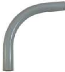
PVC Conduit Elbow or Sweep It has a long radius and is connected by gluing couplings on elbow and pipe.
