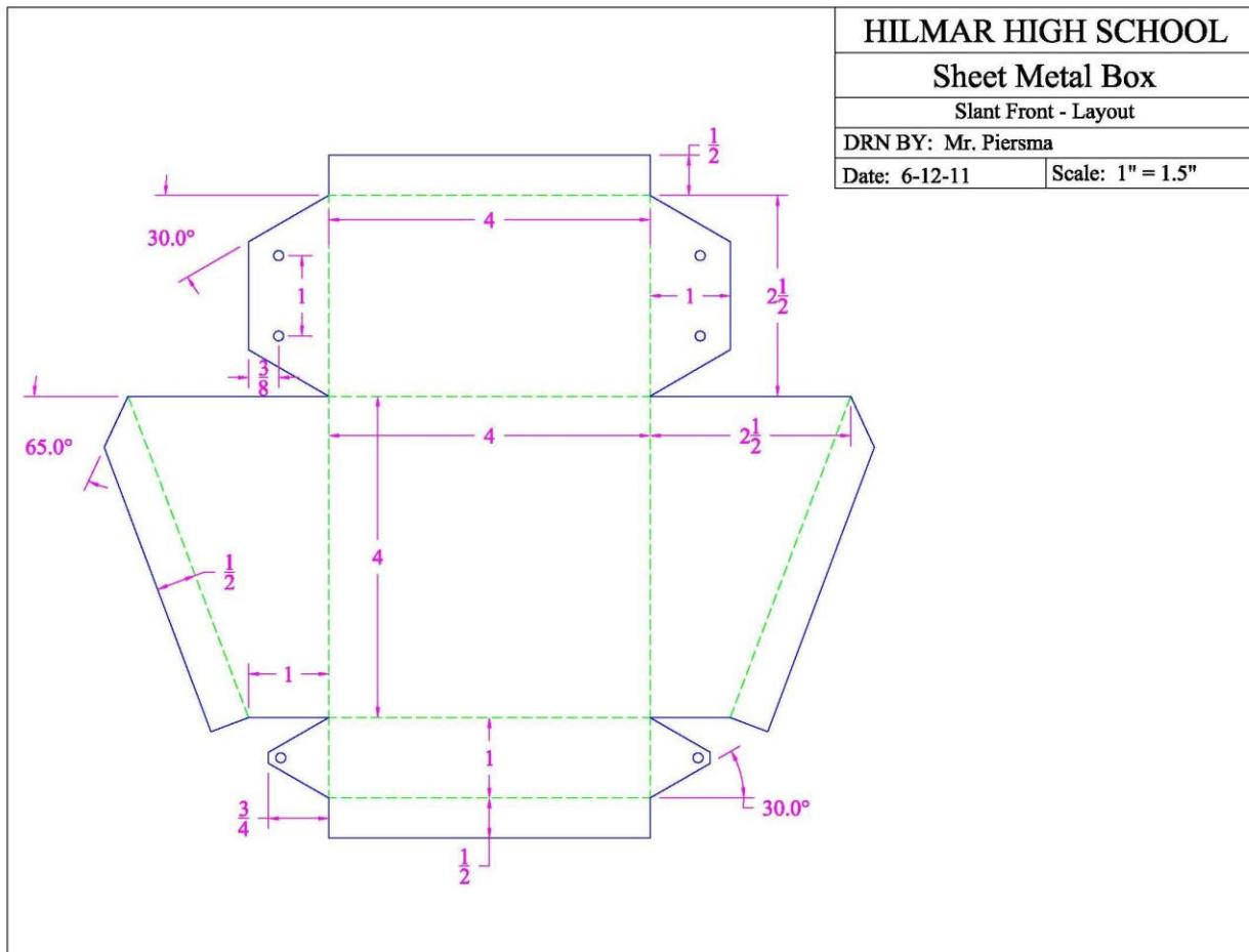
2. Using a file folder and sharp pencil layout the project shown above using the procedure described.
