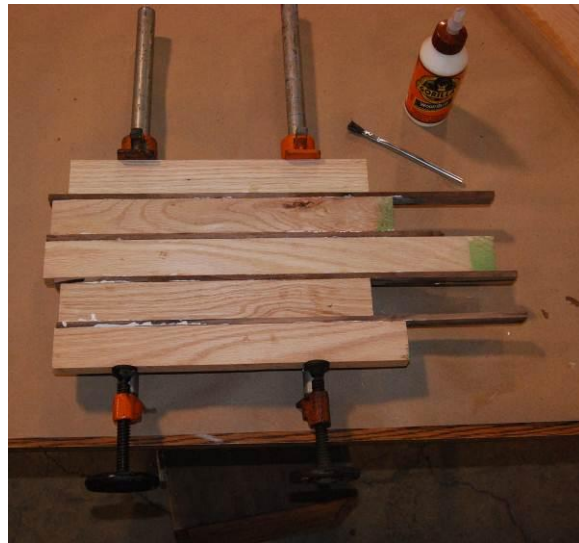
Gluing in pipe clamps
